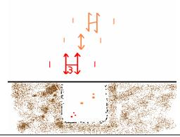
Multiple cables same trench. Staggered marks for different Utilities. Lightning bolt for CATV.
