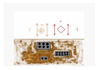
When multiple structures are known to be on top of each other the # will be placed inside the Diamond .
