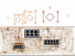
Multiple Duct Structures Marked out separately with Utility ID and Proper Color Orange Telecommunication Red Electric
