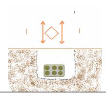
2 Single Double ended Arrows With a Diamond in between. This mark will be on any Multiple Duct Structure
