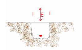
A Single Double Ended Arrow on the ground for a SINGLE cable or wire below.
